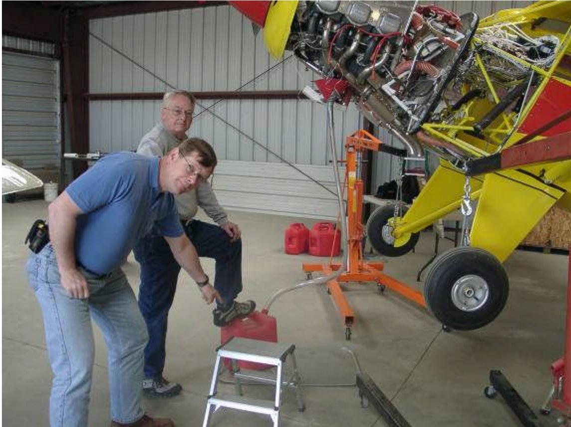
After the test was completed, the pitch angle was checked again to determine if the cranes had leaked down significantly. Strangely enough, the pitch angle had increased (!) by 0.1 degree. This was suspected to be because of the reduced weight (unlikely) or experimental uncertainty (more likely).
