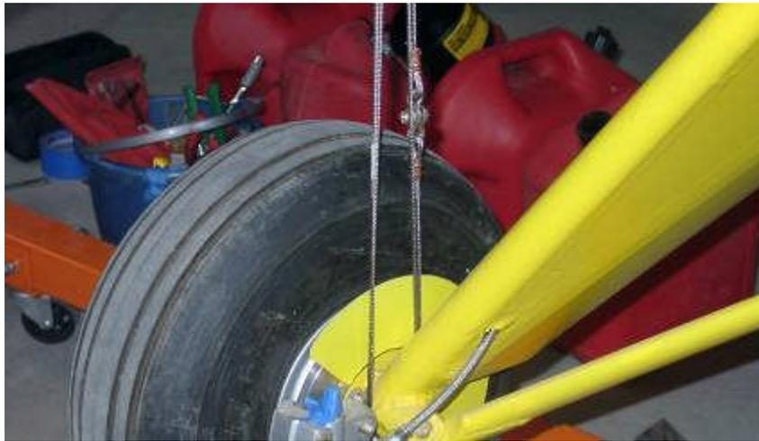
As shown here, the cable was formed in a double loop. This reduced the load on each strand by half of what the load would be for a simple loop. The picture above shows on double loop cable. This was from a previous attempt. For the lift, two independent double loop cables were used on each side. If, for some unforeseen reason, one cable was cut or otherwise broke, the other cable would support the axle long enough to get the tires back down to the floor.
