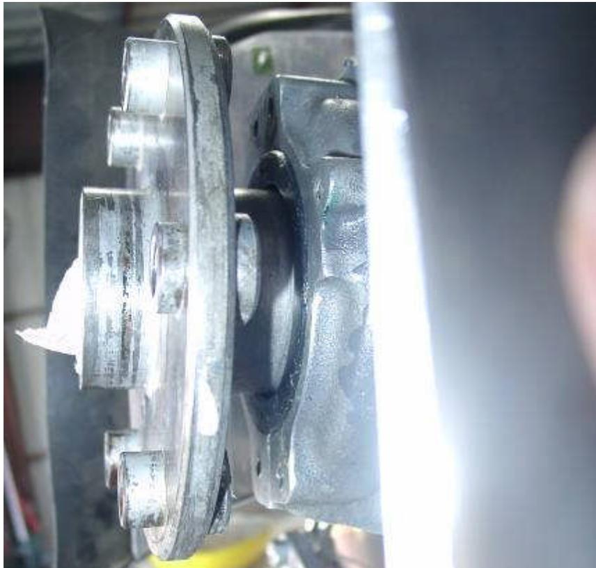
It turns out that when the Lightspeed direct crank ignition pickup board was reinstalled, the bracket overlaps part of the seal and helps to retain the seal.
