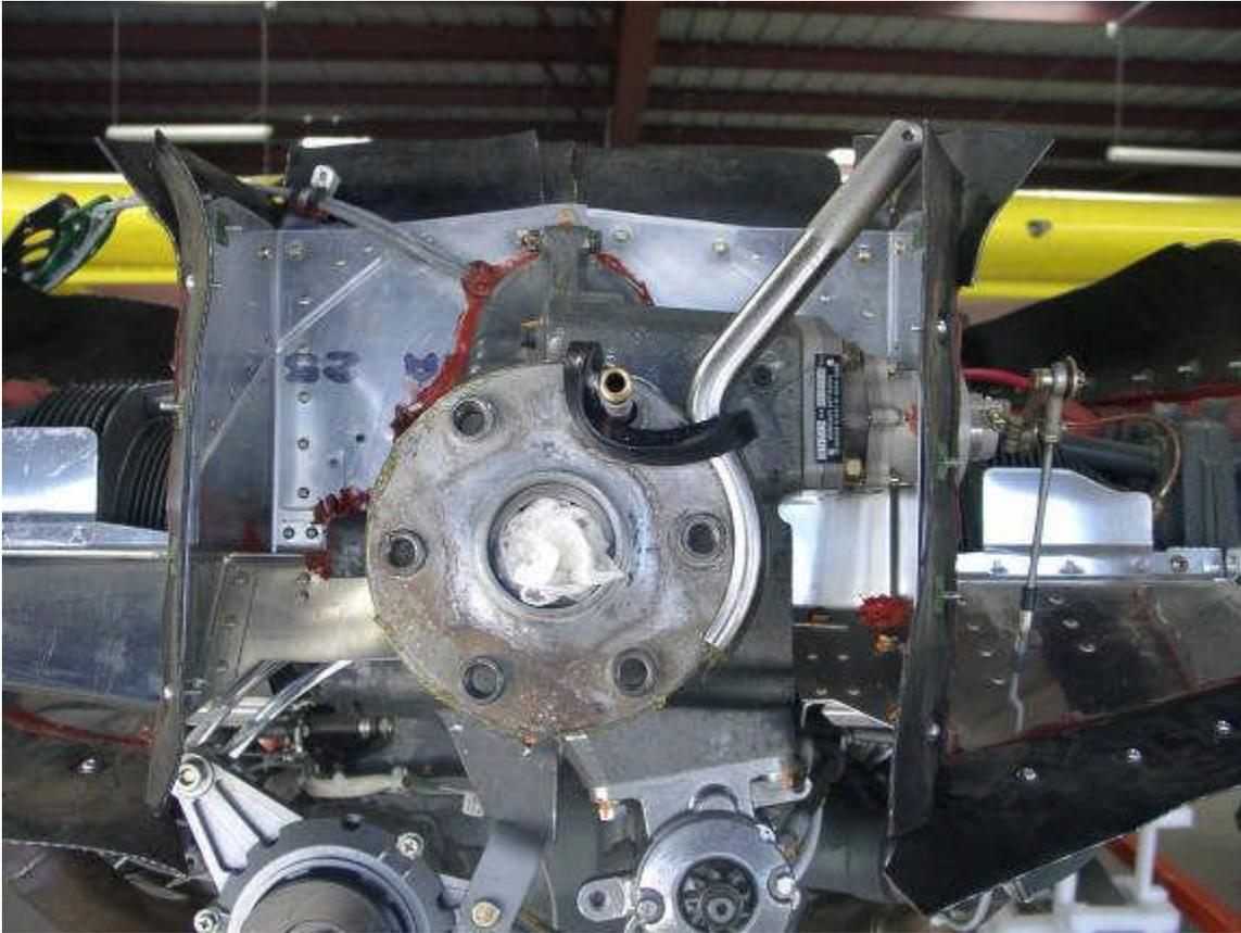
Using the tool, the seal was stretched around the prop flange by pulling the tool around. At this point, the seal sat happily around the crankshaft. The spring was wrapped around the crankshaft, hooked together, and worked back into the slot in the seal.
