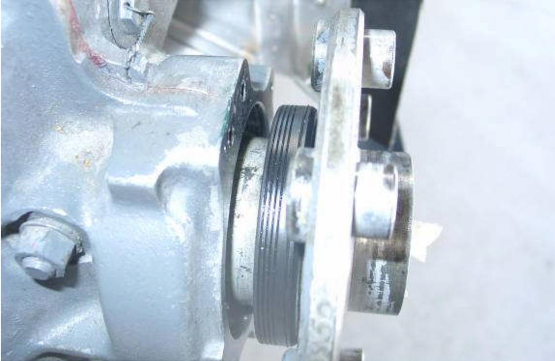
“Pliobond” cement (Aircraft Spruce P/N 09-28000) was applied around the circumference of the rubber seal and the seal was pressed into the cavity.
