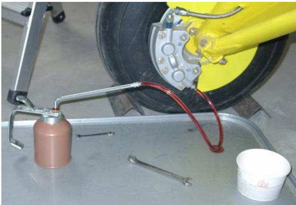
I filled the right side system first, mostly because that was the side I was standing on when I was ready to start. The first few pumps were back into the ATF bottle until the plastic tube was filled with fluid with no air bubbles. It took 60 pumps to fill the system, as indicated by fluid appearing in the reservoir. A wooden mixing stick (sold as a tongue
