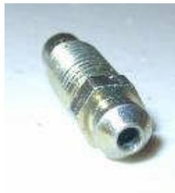
The open end shown here is where the fluid comes out or goes in depending on which direction you're pushing it. The plastic tube will slide over this end. The hex area takes a 1/4" wrench to tighten or loosen the bleeder valve.
