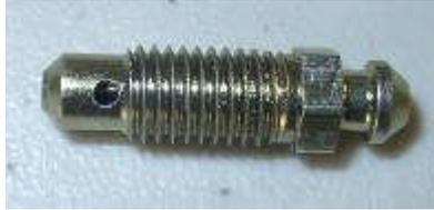
The hole at the left end is connected to the hole at the right end. As done here, the fluid is forced in the right end, comes out the hole on the left, and continues on into the brake assembly.
