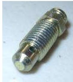
The end shown here is the interior end. The conical portion presses against a seat in the brake assembly and forms the seal that keeps the brake fluid in the system when the bleeder valve is screwed all of the way in.
