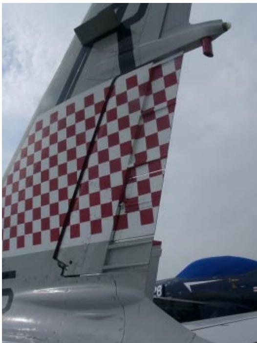
Photo-4 Rich Sugden's FJ-4B With "Splitter" Rudder (Russ Erb)
