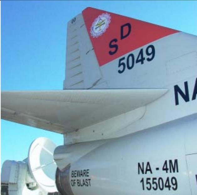
Photo-3 Note Increase Thickness At Rudder Leading Edge (Toby van Esselstyn)
