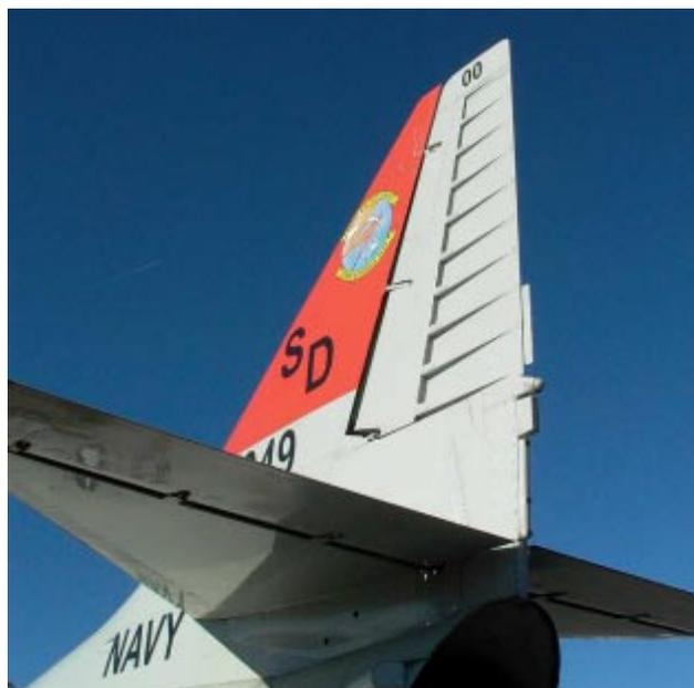
Photo-2 The A-4 Unique Rudder Design
