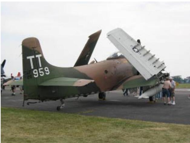
The A-1 Skyraider—the only single seat aircraft big enough to have a DOOR in each side of the fuselage
