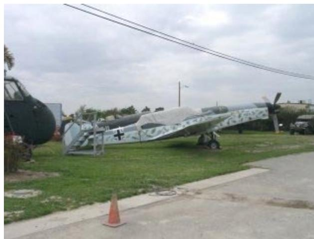
This aircraft was photographed at the **Planes Of Fame** in Chino. Per the sign, this is a **Fabrique Federale Farner-Werk C-3605 Schlepp** (you knew that, right?). It was "originally designed in the 1940s as an attack fighter with an inline engine. In the late 60s, 23 were re-engined with turboprop engines and used as target tugs. They flew with the Swiss Air Force well into the 70s."
