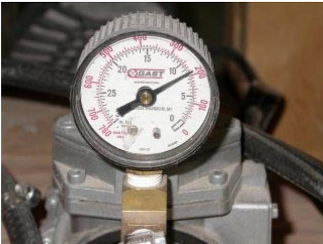
**Pressure gauge on the Suckinator, showing about 8.5 psig vacuum**
