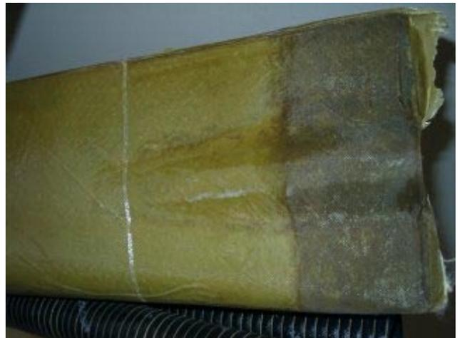
Close up of wing tip surface. Note resin ridges from where the bag wrinkled. These will need to be sanded off
