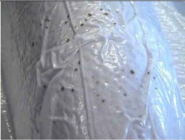
**The specks on the Speckled Trout start to appear as the vacuum reaches -8 psig. Note the wrinkles in the bag—these will lead to resin ridges requiring sanding off later**
