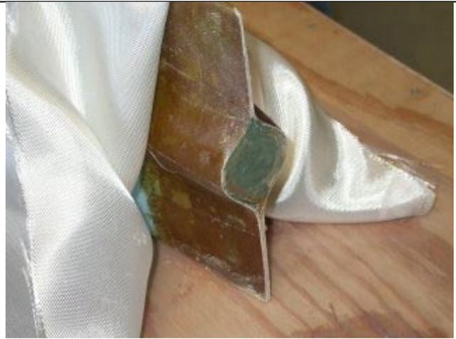
**Modeling clay was packed into the aft position light cavity to keep resin out of the screw holes and keep it easy to dig out the foam underneath**
