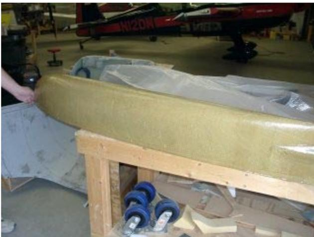
Surface of the wing tip after removing the peel ply and associated bagging materials
