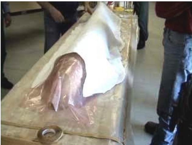
**The breather applied over the perf ply. The breather material is essentially the same as batting used in making quilts. Its purpose is to provide an air path between the perf ply and the plastic bag and to absorb the excess resin**
