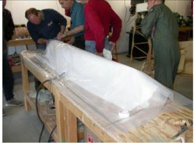
**The bag is wrapped around the alien, and the top sheet is carefully pushed down into the sealing tape**
