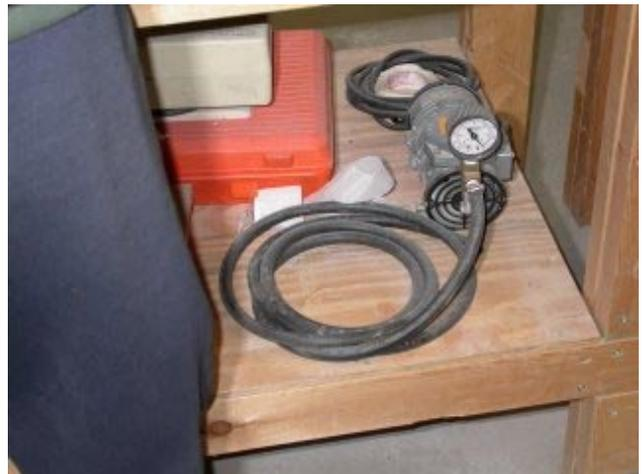
**The vacuum pump, aka "Suckinator," stands by ready to remove the excess air. A bleed valve allows setting the vacuum pressure drawn**
