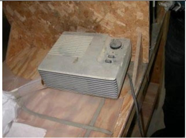
**The heat source, an electric space heater specially modified by Waldo to allow it to run at higher temperatures without cutting out**
