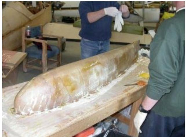
**The peel ply is sliced as required and squeegeed into the resin. No resin is added, but the extra resin starts to wick up through the peel ply**
