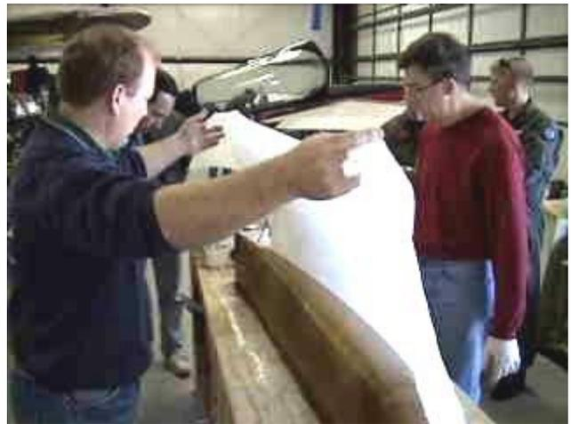
**The peel ply is applied. This Polyester (Dacron) fabric has a very low peel strength with the epoxy, allowing the vacuum bagging materials to be separated after the epoxy has cured**
