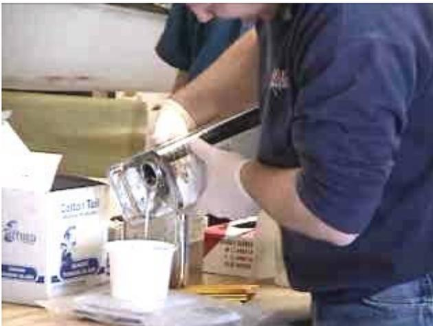
**Note the Professor's technique. By pouring the resin in this fashion, more of it goes in the cup and less ends up on the outside of the can**
