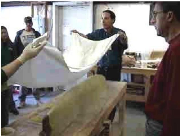
**The Master directs the application of the first layer of fiberglass cloth**
