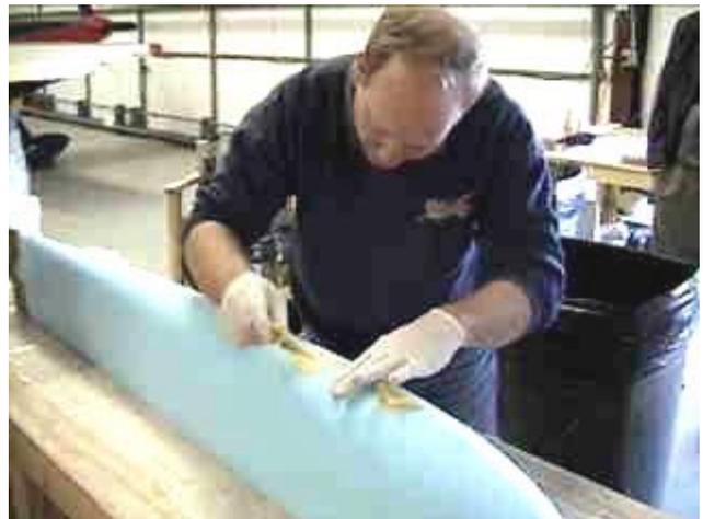
**Professor Waldo spreads the peanut butter consistency micro into the divots at the end of the tips. Because the microballoons are filled with air, this mixture is much lighter than epoxy resin alone**
