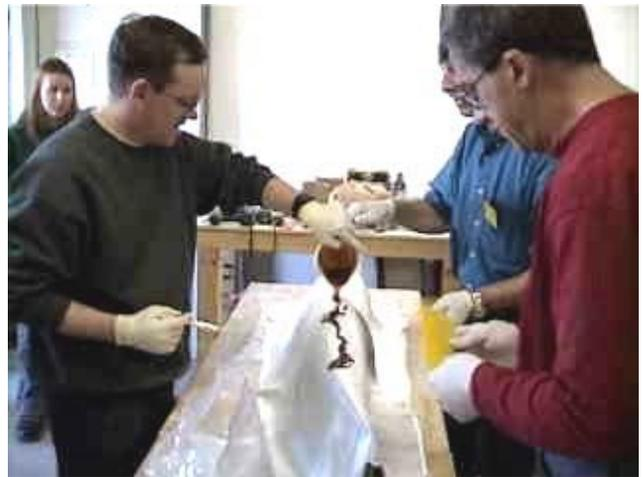
**Applying the initial slug of resin**
