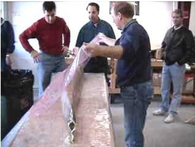
**With the "part" resting on one side of the vacuum bag, Professor Waldo applies the perforated release sheet. This plastic sheet has small holes in it to allow the excess resin to pass through into the breather**
