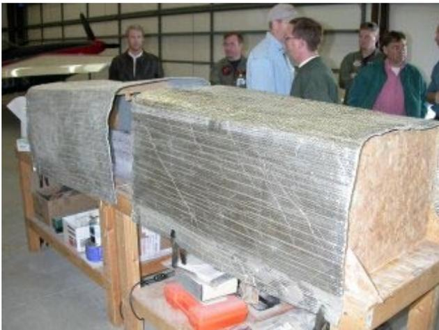
**Preparing the heat tent. With the ambient temperature hovering around 59° F (15° C), the epoxy does not flow as well (higher viscosity) and takes longer to cure. This simple heat tent fixes both problems**
